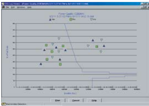
ITIC/CBEMA Plotting showing damaging Power Quality events.
