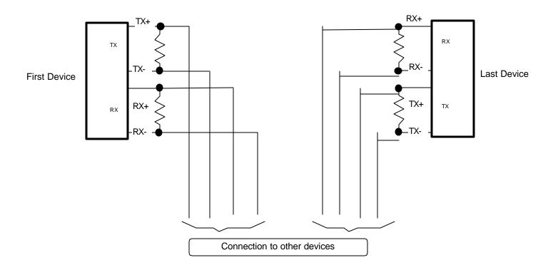
Fig.1 Full Duplex installation with terminating resistors.
