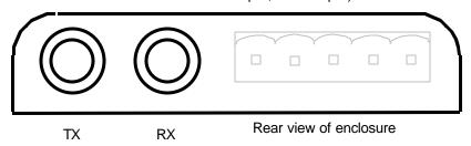
Power Connection: DC Jack barrel type (not polarized)
