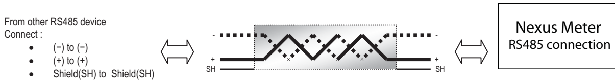
Figure 5.5: 2-Wire RS485 Port Detail
