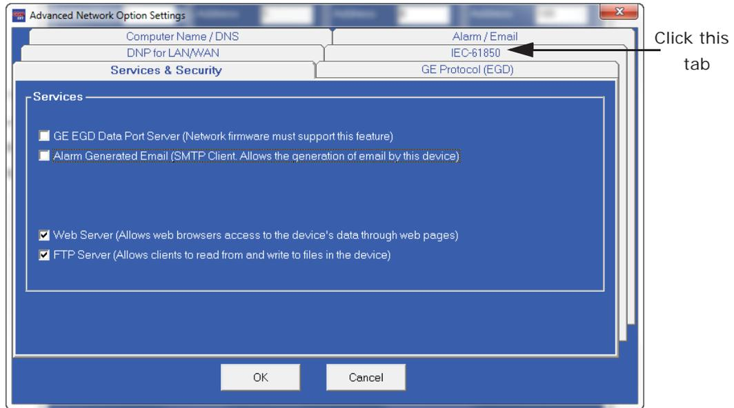
5. Make sure the checkbox to enable the IEC 61850 Protocol Network server is selected, as shown below.
