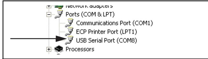
In this example, COM8 is the Virtual port: COM8 is the port you select in the Connect screen.
