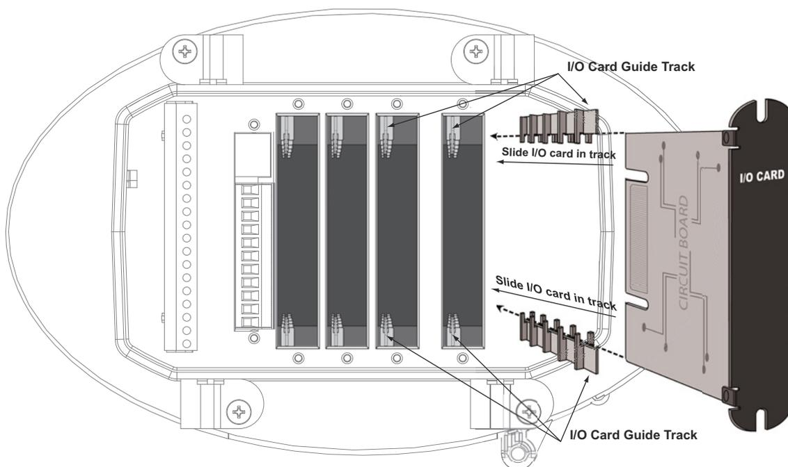
Figure 11.1: Inserting an I/O Card into the Meter
