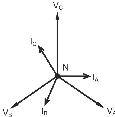
Figure 1.2: Phasor Diagram Showing Three-phase Voltages and Currents
