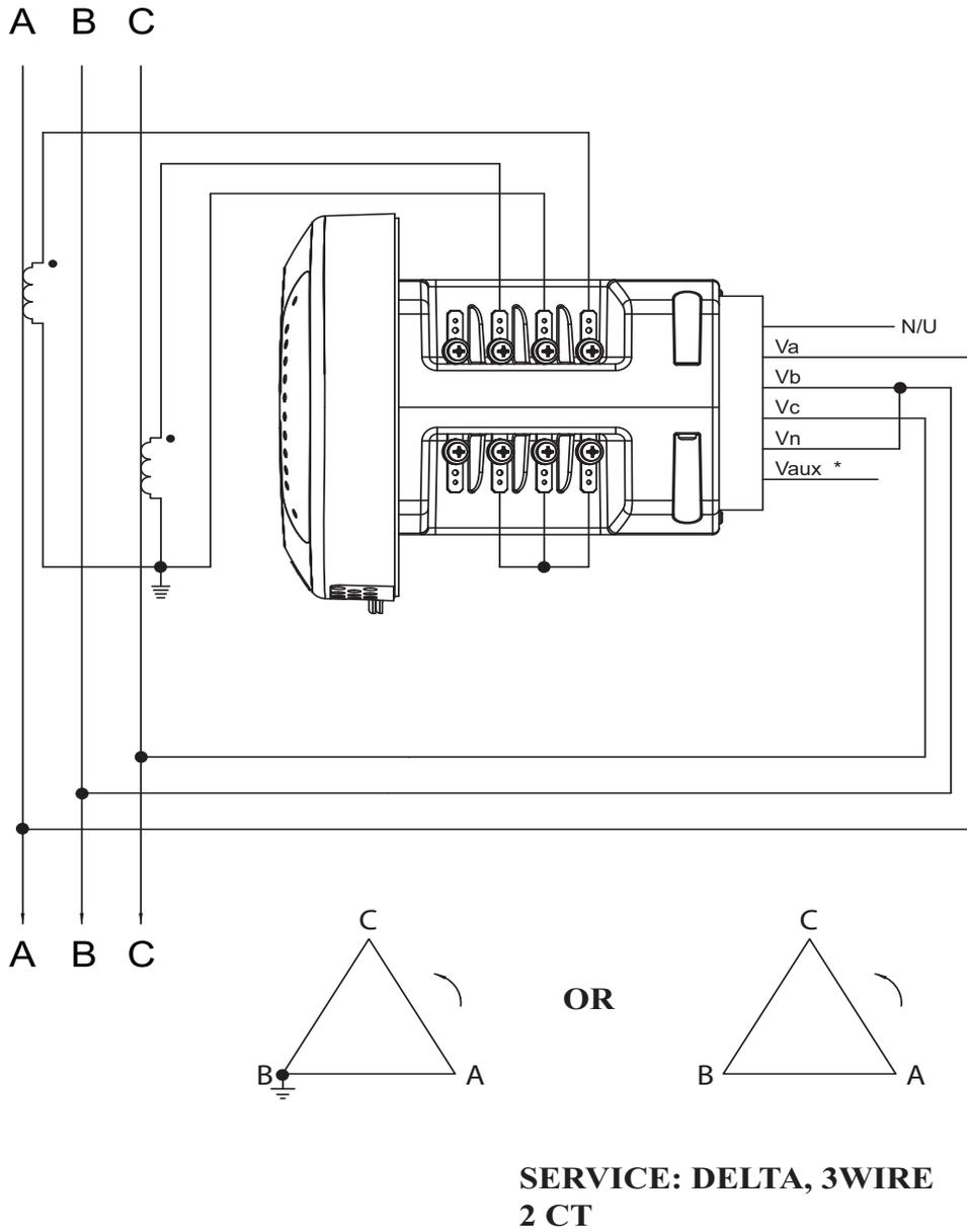
Figure 4.10: 3-Wire, 2-Element Open Delta Direct Voltage with 2 CTs
