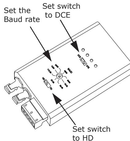
com's Baud rate must match the Baud rate of the meter's RS485 port: you set the Baud rate by turning the screw to point at the rate you want.
