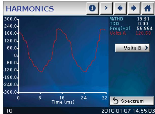
Touch **Volts B** to view the Harmonics screen for Phase B - N voltage; Touch **Volts C** (from the Volts B screen) to view the Harmonics screen for Phase C - N voltage.
