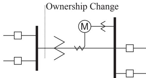
Figure 7.1: Low Voltage Metering Installation Requiring Loss Compensation
