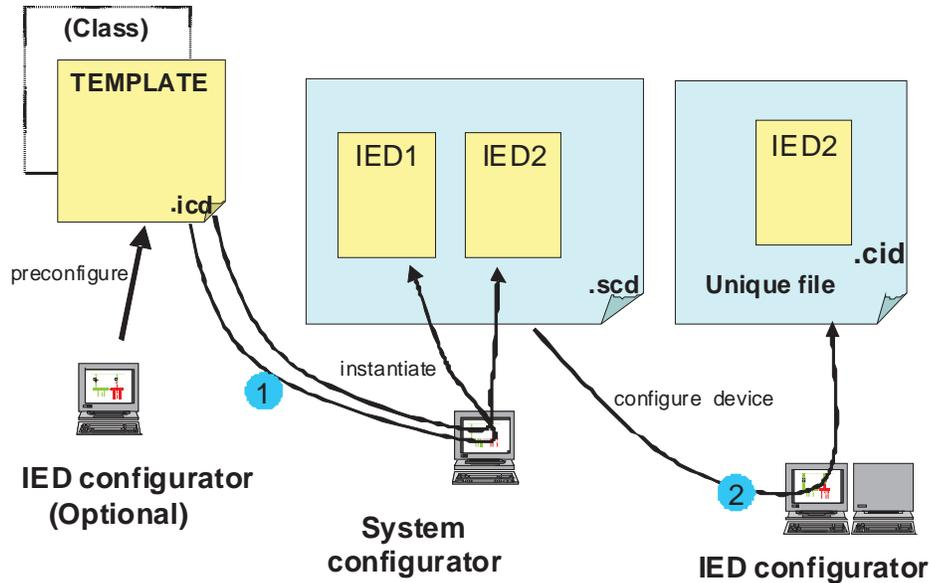
Figure C.2: Configuration Process
