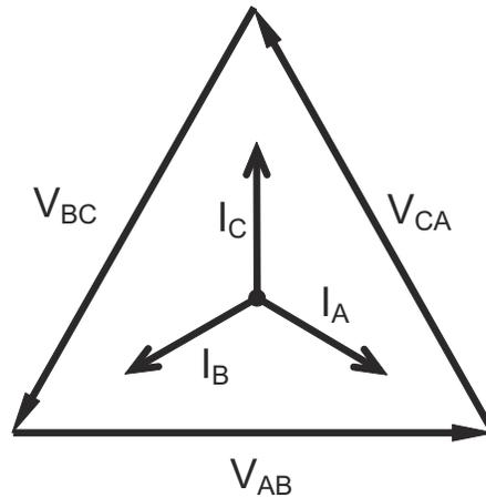
Figure 1.4: Phasor Diagram, Three-Phase Voltages and Currents, Delta-Connected
