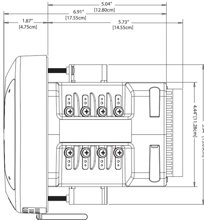
Figure 3.2: Meter Dimensions (Top and Side)
