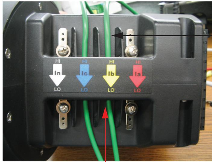
CT wire passing through meter with current gills removed
