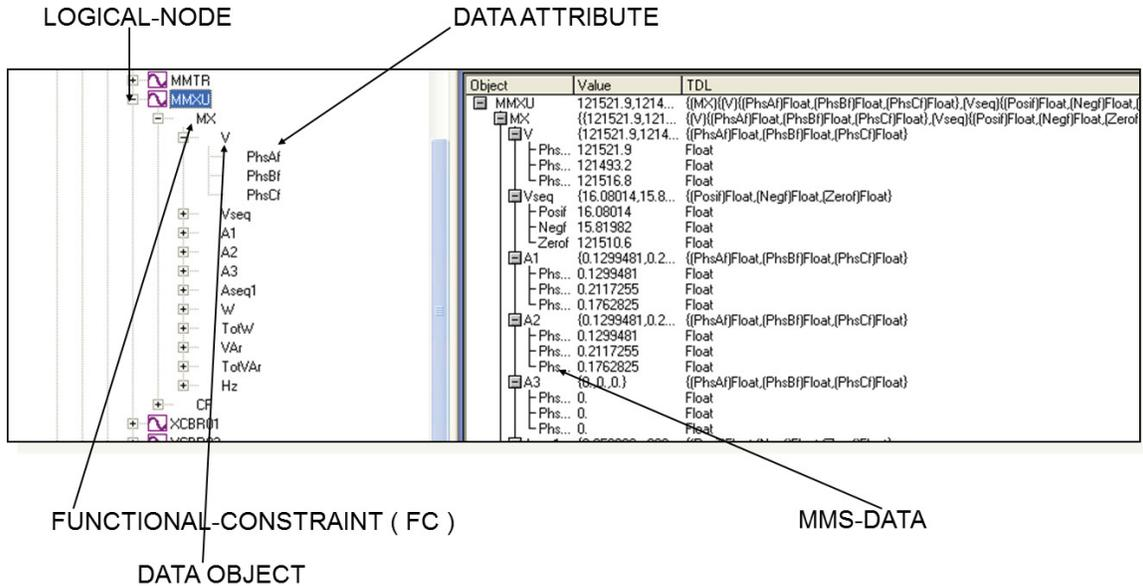
Figure C.1 Object Model Display on a Diagnostic Browser
