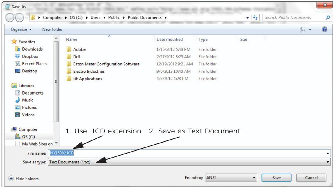
12. Once the System Integrator has processed the Nexus® 1500 meter's .icd file and the information of the other devices on the network (using either automated tools or manually), the final result is a configuration file with the extension ".cid". This file must now be uploaded to the Nexus® 1500 meter's IEC 61850 Protocol Ethernet network card.
