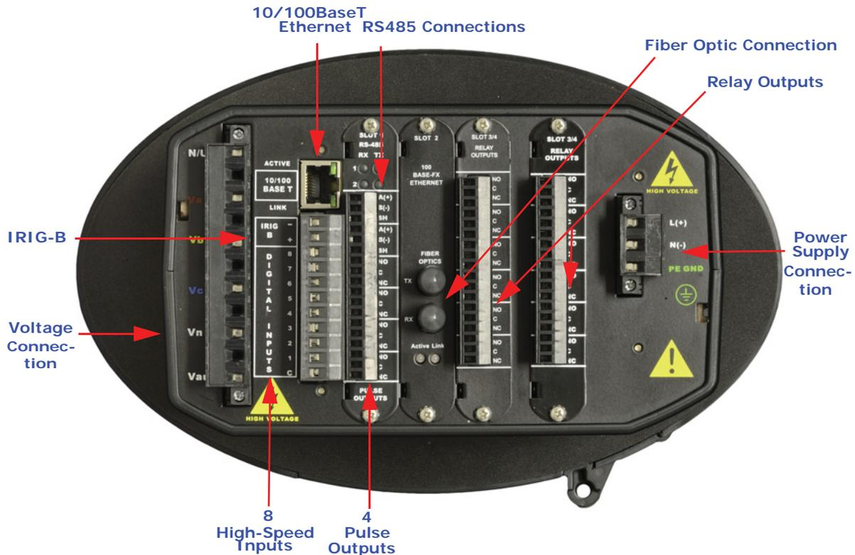
Figure 4.4: Voltage and Power Supply Connections, RS485, Pulse Outputs, IRIG-B, 10/100BaseT Ethernet, High-Speed Inputs, Fiber Optic Connection, and Relay Outputs
