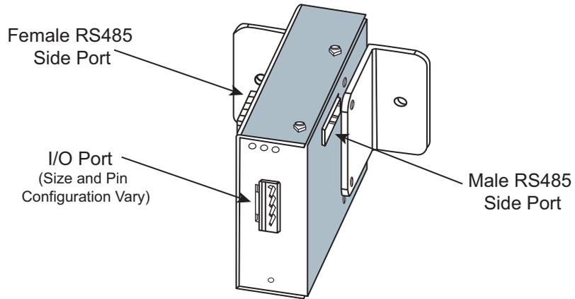
Figure 3.6: External I/O Module Communication Ports and Mounting Brackets
