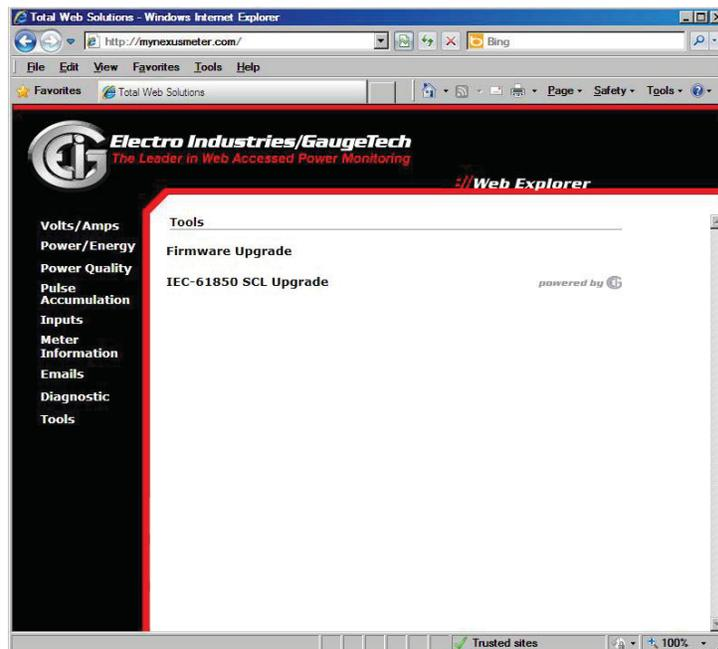
To upgrade the meter's firmware, click **Firmware Upgrade**. See Appendix C for details on the IEC-61850 SCL Upgrade option.
