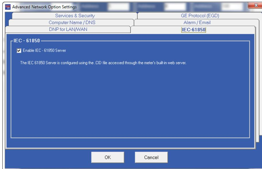
6. Click OK and then click Update Device to send the settings to the Nexus® 1500 meter. The meter will reboot. The IEC 61850 Protocol Ethernet Network server is now configured properly to work on an IEC 61850 network.
