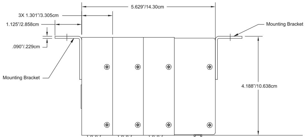
Figure 3.7: External I/O Modules Mounting Diagram, Overhead View
