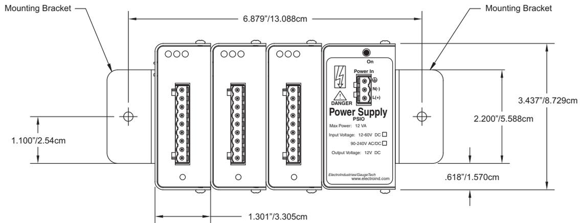
Figure 3.5: External I/O Modules Mounting Dimensions, Front View
