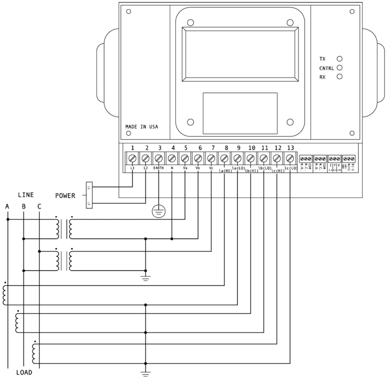
**III. Three-Phase, Three-Wire Open Delta with three CTs and two PTs.
