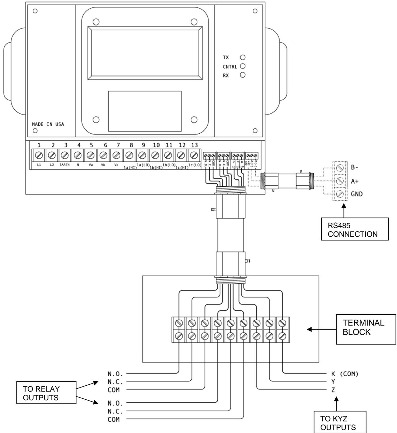
**Figure A-3.1:** Wiring Diagram of DMMS 300B
