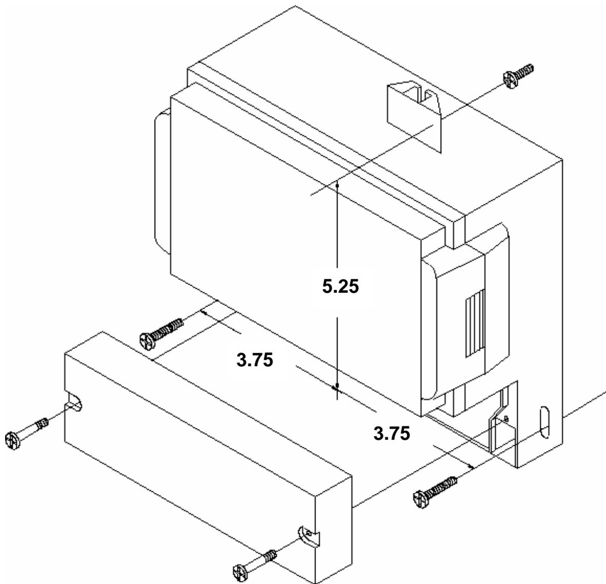
**Diagram A-1.2** Mounting Detail for DMMS B.
