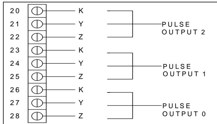
**Figure A-2.1:** KYZ Relay Connection for NL2 Option
