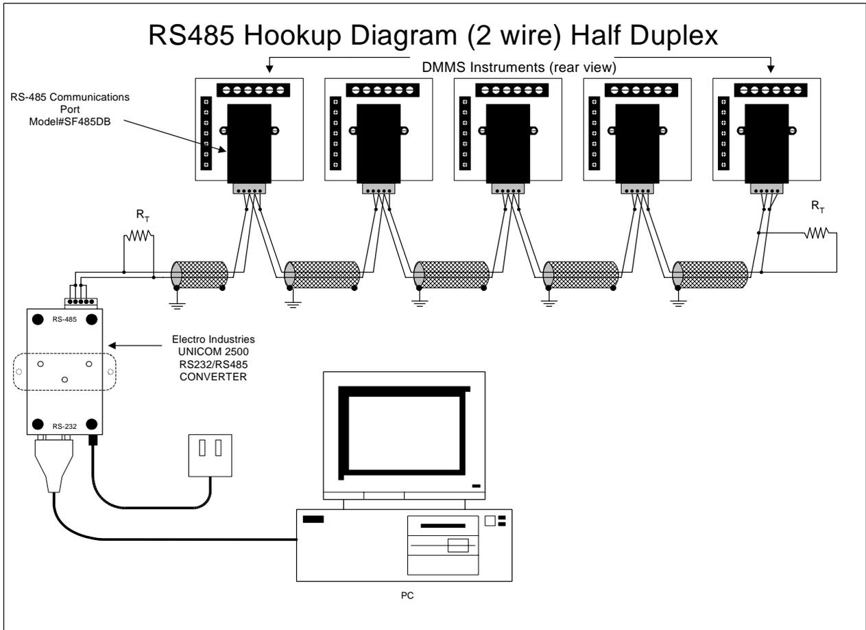
**Figure 4.2:** 2-Wire RS485 Communication Connection Installation half duplex
