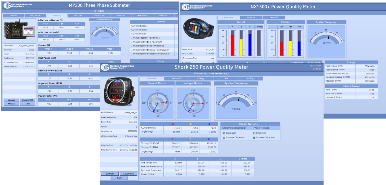
Real Time Electrical Usage Dashboards for Installed Power and Energy Meters
