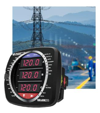
The Shark<sup>®</sup> 250 is an ANSI C12.20 0.1 Accuracy Class meter that provides highly stable, precise, and reliable measurements that maintain accuracy over time. It has comprehensive revenue energy measurement capability, including CT/PT compensation, test mode and energy presets, pulse accumulators and totalizers, and up to eight pulse outputs/inputs. It is field upgradeable and offers multiple I/O and communication capabilities.
