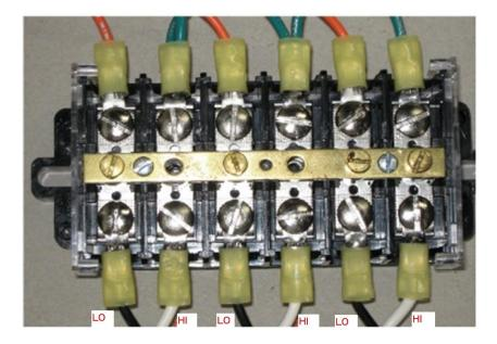
In most split core CTs, the polarity lead is white or red and the non polarity lead is black (see the figure on the previous page). In the solid core CT, the secondary terminals are marked as X1 for the polarity terminal and X2 for the non polarity terminal. Sometimes, only X1 is marked, as shown in the figure below.
