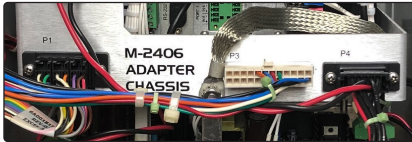
Figure 19 M-2406 Adapter Chassis P1, P3, and P4 Connectors (14- / 19-pin Adapter Chassis Shown)
