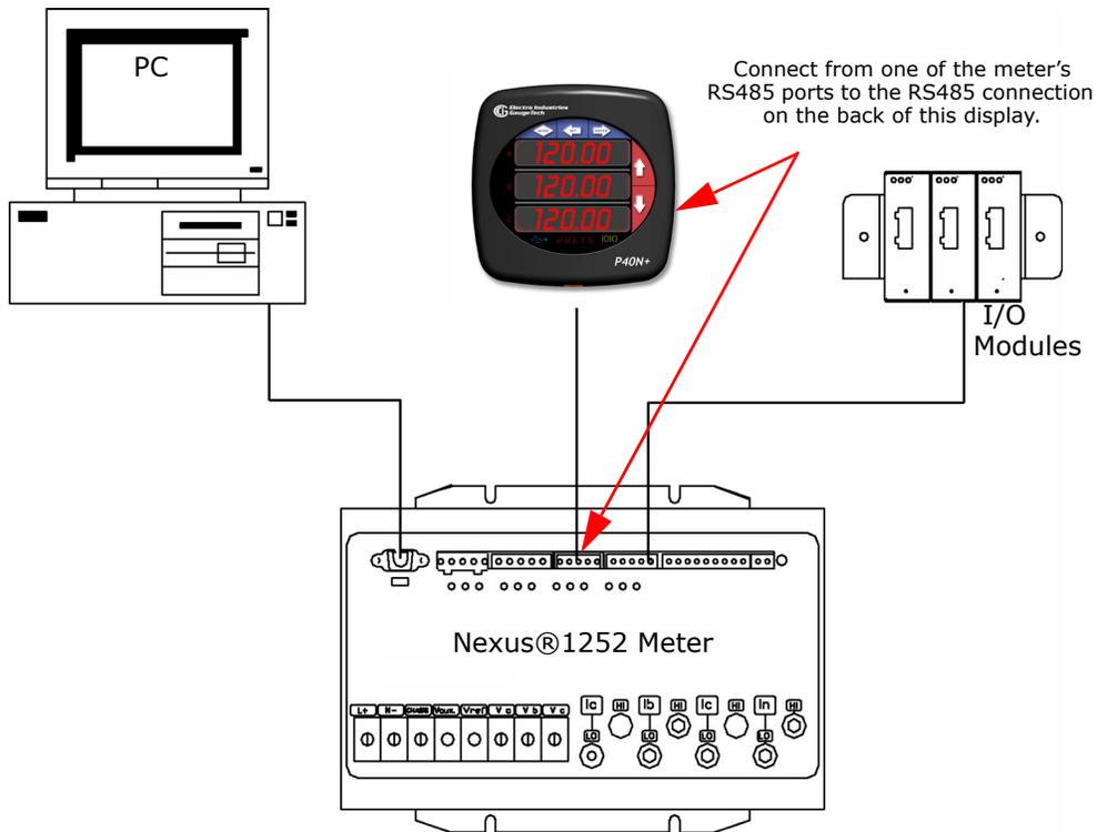
**Installing an External Display:**
