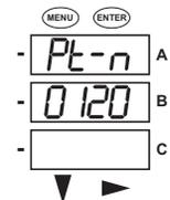
7. Press the **ENTER** button to go to the PT numerator setting screen (Pt-n). The current PT numerator is shown in the second line. To change the setting, press the **DOWN ARROW** until the value you want is displayed. Then press the **RIGHT ARROW** to move to the next digit. Repeat until the setting is done.
