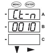
5. Press the **ENTER** button to go to the CT denominator screen (CT-d). This setting is display only - it can't be changed.
