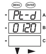
8. Press the **ENTER** button to go to the PT-denominator screen (Pt-d). The current PT denominator is shown in the second line. To change the setting, press the **DOWN ARROW** until the value you want is displayed. Then press the **RIGHT ARROW** to move to the next digit. Repeat until the setting is done.
