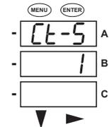
6. Press the **ENTER** button to go to the CT Scaling setting screen (CT-S). The current Scaling is shown in the second line. Press the **DOWN ARROW** to choose another value. You can choose 1, 10, or 100.
