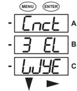
11. Press the **ENTER** button four times. (You will pass through the Address, Baud Rate, and Protocol screens. **You DO NOT change any of the settings on these screens.\*\***You will see the Scroll setting screen (SCrL). The current setting is shown in the second line. Press the **DOWN ARROW** to choose another setting. You can choose YES (the meter readings will scroll on the display) or no (the meter readings will not scroll on the display).
